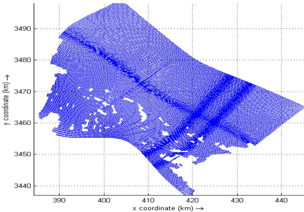
**Figure (1) Computational Grid of the Flow Model of the Lake**
